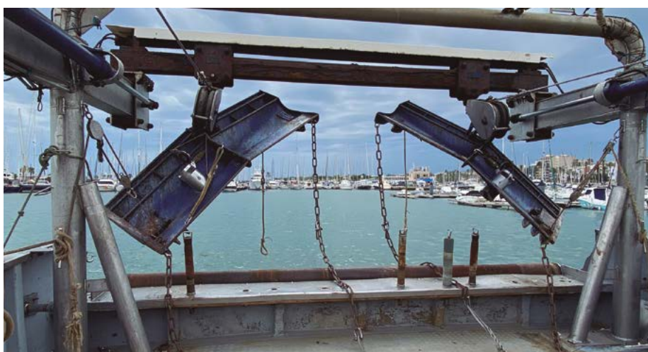
Doors without contact with the sea bottom in trawling mode. Source: General Directorate for Maritime Policy and Sustainable Fisheries.
