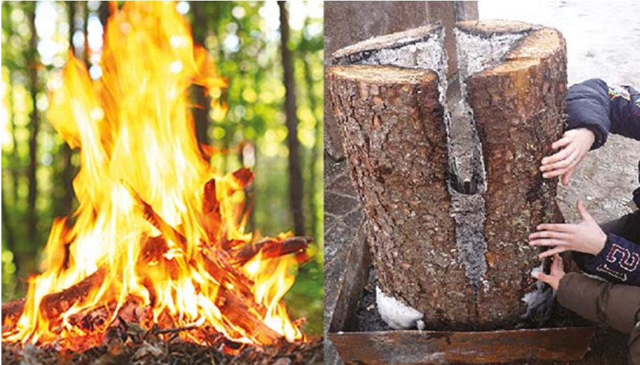
Figure 2. Wood burns more or less easily depending on the mass of the element. Photos: Timber fire behaviour. Roberto Tomasi. Lund University.
