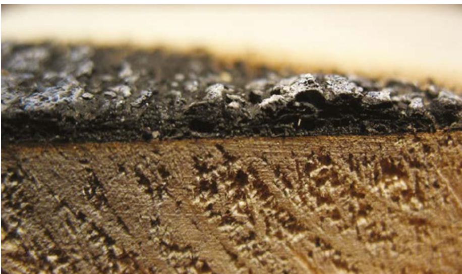
Effect of an intumescent paint in contact with fire. Photo: Teknos
