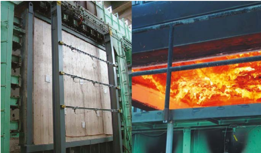
Figure 4. Tests of CLT cross-laminated timber panels. Photos: FP Innovations Canada.
