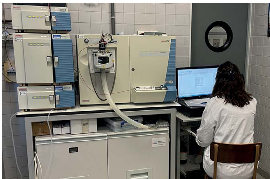
Electrospray ionisation source and ion trap mass spectrometer. Photo: ChroMS-EnviFood.
