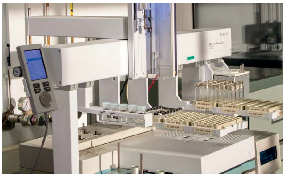
Gas chromatograph with single quadrupole mass spectrometric detector. Photo: AFL
