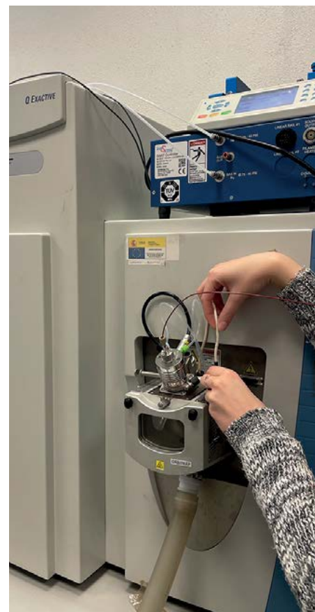
LC-HRMS: Atmospheric pressure chemical ionisation source (APCI) and hybrid quadrupole-Orbitrap mass spectrometer. Photo: ChroMS-EnvFood.
