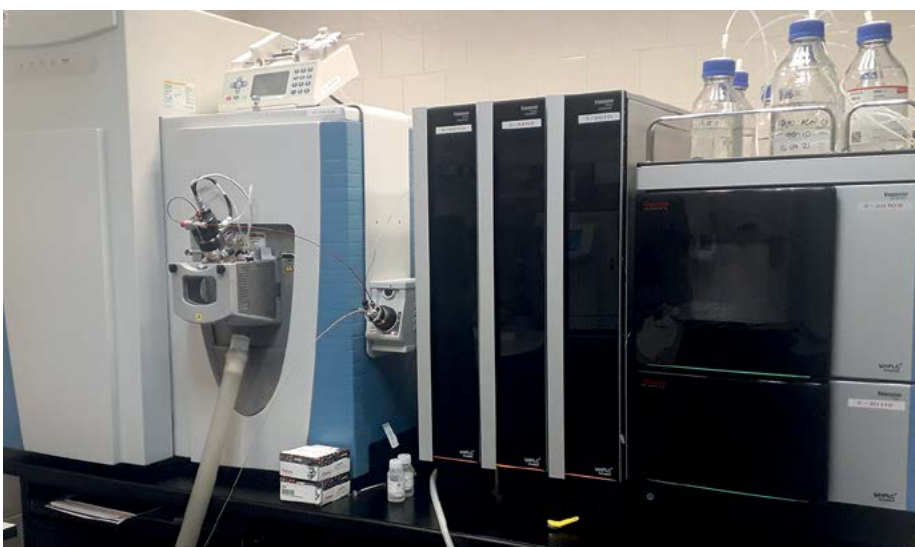
Liquid chromatograph coupled to high resolution mass spectrometry (UHPLC-HRMS). Photo: Barcelona Public Health Agency
