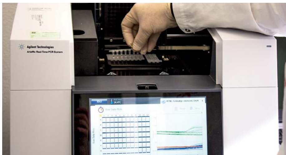
Loading of samples into a real-time thermal cycler. Photo: AFL
