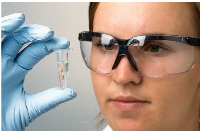
The tube held by technician Sheri Mazenko contains concentrated immunomagnetic beads coated with antibodies that bind to specific bacteria, making it possible to detect contaminants in food.
