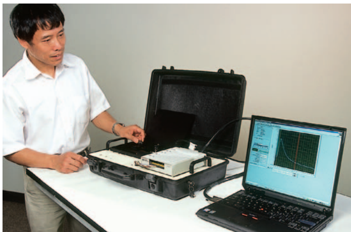
Chemist Guoying Chen tests a portable fluorometer he designed and built to screen for drug residues in food extracts.
