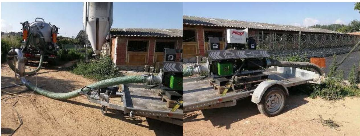
**Figure 1.** Photo of the sampling equipment connected to the tank and the NIRS (left) and the stationary equipment (right)
