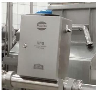
Figure 1. Meat emulsion sensor installed on the Frankfurter sausage production line at the homogenizer outlet
